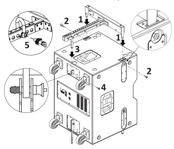
Please note that the Rear Link Bar of the SW215FAV2 cabinet has two holes (see figure): The hole signed as **nr.1** must be used for **SW215FAV2-SW215FAV2** sub-sub link. The hole signed as **nr.2** must be used for **SW215FAV2-AX2065** sub-sat link.
