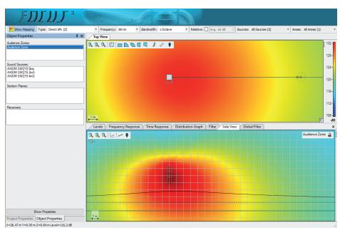
NOTE: in this figure is shown the result of an suspended array with each box delayed of 2mS progressively, this method point downward the wave propragation to avoid roof reflection at 80Hz octave.
