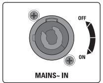
**MAINS IN** - Powercon® NAC3FCA power input connector (blue). To switch the amplifier on, insert the Powercon® connector and turn it clockwise into the ON position. To switch the amplifier off, pull back the switch on the connector and turn it counter-clockwise into the POWER OFF position.
