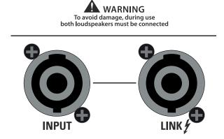
**LINK** - Power output in parallel with the INPUT socket for connecting the unit to another speaker. The number of SW218P cabinets that can be connected in parallel depends on the amplifier load capacity.
