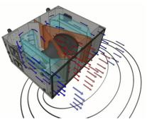
transmission line paths as well. Its working principle is an hybrid combination between a short transmission line and an overdamped reflex load. Moreover, the maximization of the mutual coupling between the drivers increase the fastness of the transient response while maximizing the overall energy efficiency as well.
