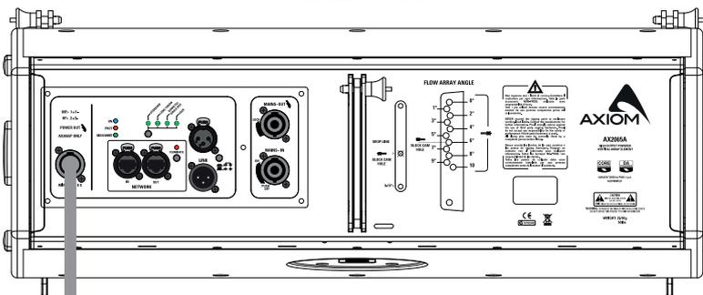
The DA module employed for powering the AX2065A delivers in an ultra-compact package a maximum power of 2000W. Moreover, each AX2065A is able to power an additional passive AX2065P module through the available power output on the back panel. This feature will allow to assemble very competitive system solutions both for rental and installation applications.
