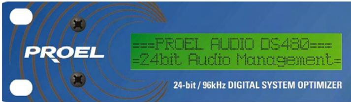
**LCD Screen:** Shows, by default, the name of the last recalled memory on the bottom line of the screen, and the current routing on the top line. Also used to show all parameters as they are edited, and all menu selections.
