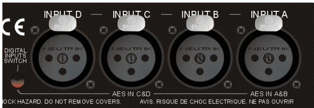
**AES Input Switch:** Recessed switch to select AES digital inputs. Red LED will illuminate in the hole when AES inputs are selected, along with the corresponding front panel indicator.
