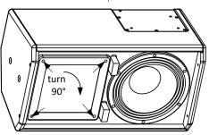
2) Unscrew the 4 screws fixing the horn and rotate the horn by 90°.
