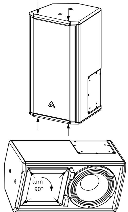
2) Unscrew the 4 screws fixing the horn and rotate the horn by 90°.
