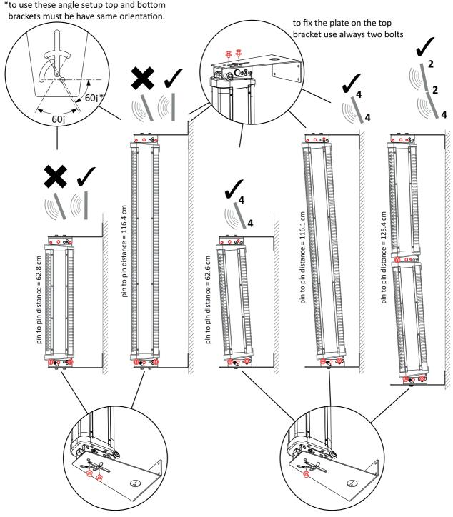
to fix the plate on the bottom bracket use two bolts (0°) or a single bolt (4° downward).
