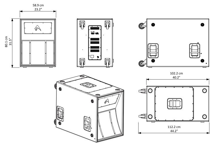
NOTE: This product is designed to work on floor and is not equipped with rigging flying points, do not suspend the loudspeakers from the handle.
